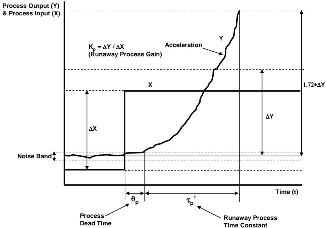
**Open Loop Runaway Response for Process with Positive Feedback**
