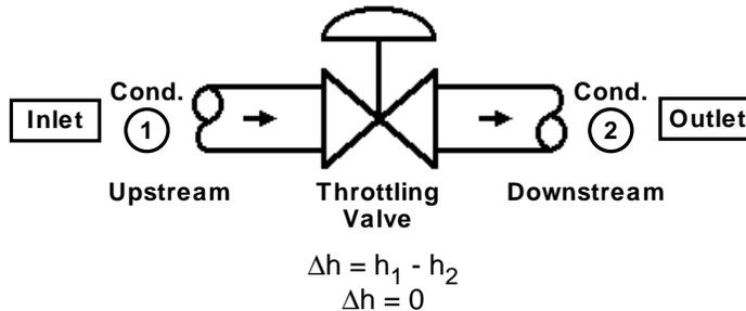
THE CHANGE IN ENTHALPY ACROSS A RESTRICTION IN A PIPE — ORIFICE, REGULATOR, CONTROL VALVE — IS “ZERO” FOR A THROTTLING PROCESS.
