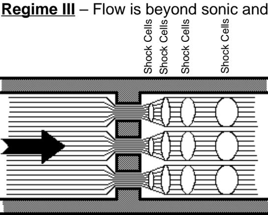
the inefficiency is such that no pressure recovery takes place. There is no clearly formed vena contracta point in the valve. There is a “strung-out”, continuous pressure drop through the valve as flow traverses. Shock cells significantly interact.
