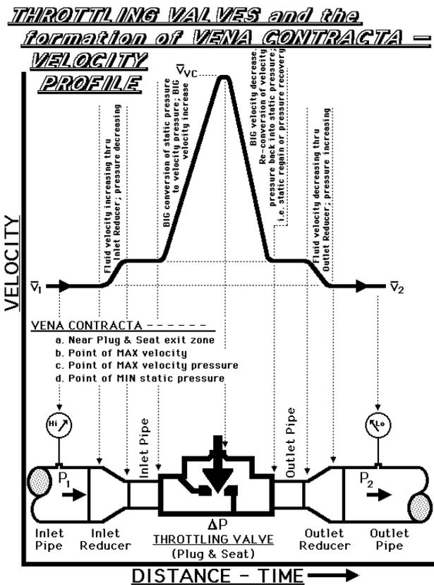
The depth of the vena contracta “dip” is primarily a function of a throttling valve’s geometry; globe vs. butterfly, etc. The important parameter in determining the  $P_{VC}$  is – “ $F_L$  – Liquid Pressure Recovery Factor”. As the name implies, the  $F_L$  factor is a measure of the effectiveness of the reconversion of velocity pressure into static pressure from the main orifice of the throttling valve (@ vena contracta) to the valve’s outlet.
