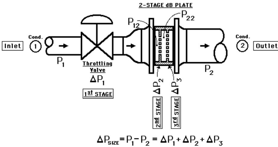
because the variable orifice(s) 1st stage throttling valve must increase its proportionate share of overall  $\Delta P_{Total}$ , as the fixed orifices dB plates decrease in their proportionate share of overall  $\Delta P_{total}$ . Such devices have a practical 4:1 turndown in flow rate to remain effective.
