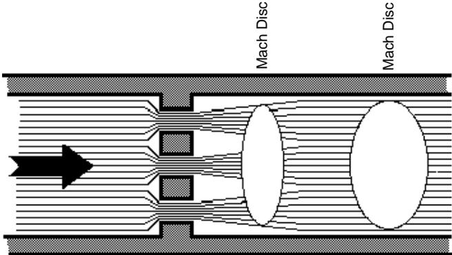
**Regime V** – In this regime the flow reaches “constant acoustical efficiency”. When in Regime V, if the P2 outlet pressure is lowered, the noise level remains constant; this would not be true in any of Regimes I through IV.
