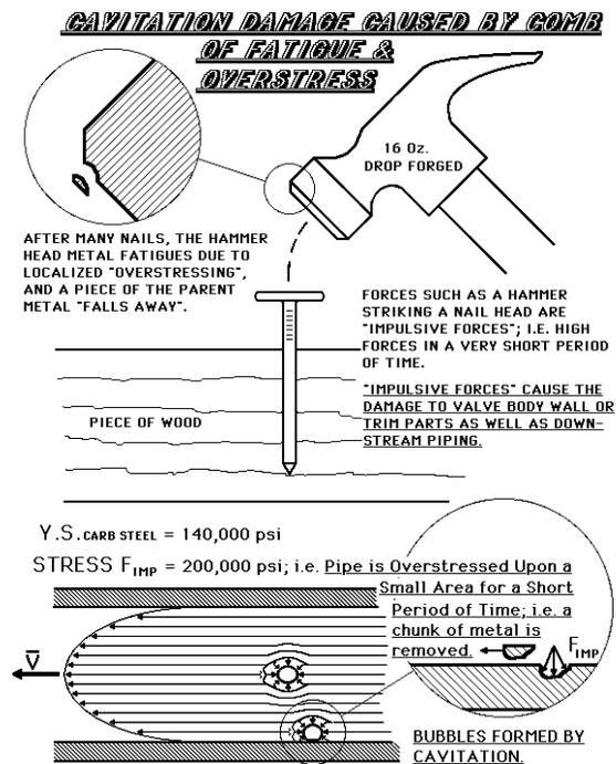
downstream piping. In reality, it creates more “expensive” problems when a fluid is in the high end of the
