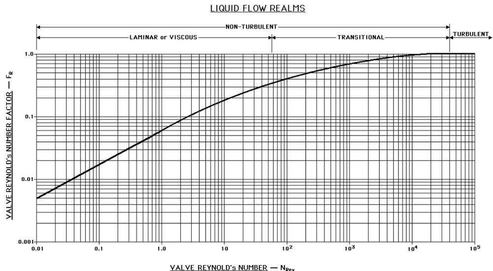
The vast number — greater than 98% — of applications of throttling valves are in the "turbulent" realm.
