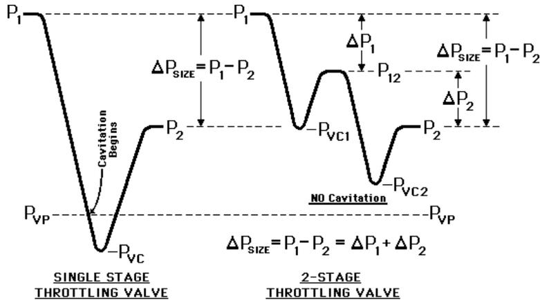
The depth of the vena contracta dip is related to the throttling valve’s “ $F_L$  factor”. Thus, simply by applying a globe or eccentric plug (rotary globe) throttling valve rather than a ball or butterfly throttling valve, you can eliminate cavitation. (See page 5.)
