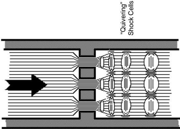
**Regime IV** – The individually formed shock cells merge together to form a single “Mach Disc”. The pressure gradient curve is similar to Regime III above. A “jump” upwards in the noise level occurs after passing from Regime III to Regime IV.
