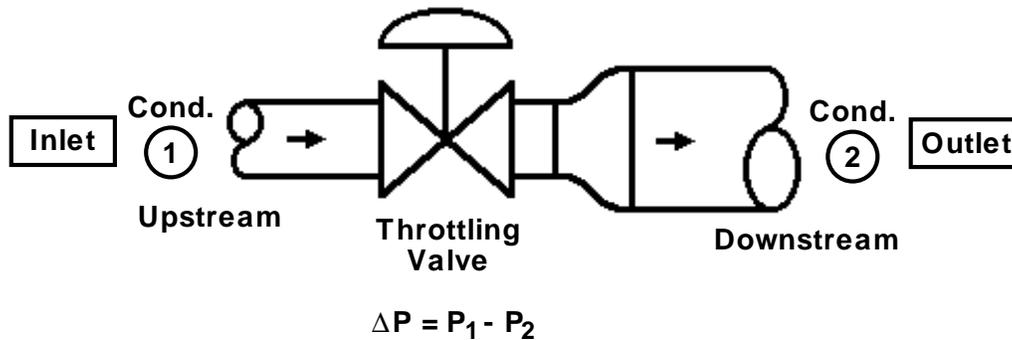
**FLOW DESCRIPTION.** Gaseous flow is “compressible flow” as previously discussed in **FLUID STATES**. This means that as the throttling valve experiences its internal pressure drop, the gas is decompressing (expanding), followed in many cases by recompression in the pressure recovery zone. Gas expansion explains why outlet pipe sizes –  $\varnothing_{2P}$  – are typically larger than inlet pipe sizes –  $\varnothing_{1P}$ ; more “space” is needed.
