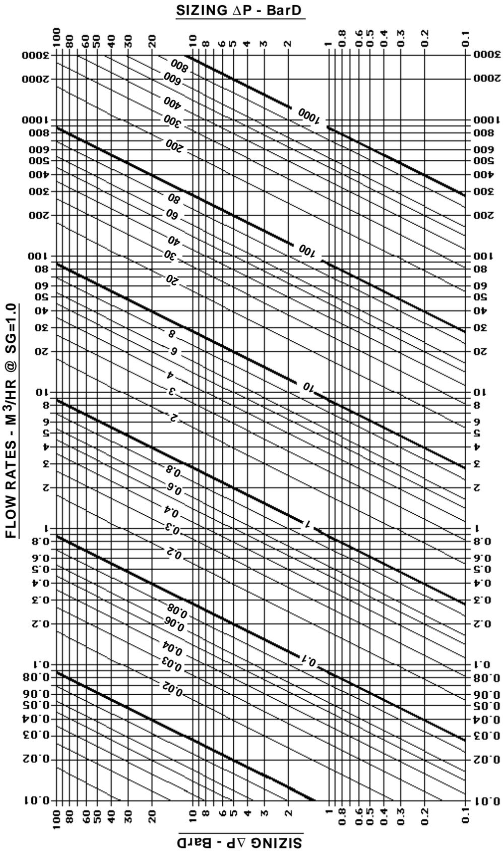
**METRIC – DETERMINING Cv FACTOR – NON-VAPORIZING \***
