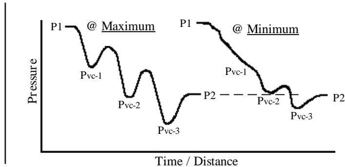
For fixed downstream orifices within a valve body, noise can be brought down to an acceptable level at maximum conditions, but as flow decreases the valve would become noisier. A reasonable rule-of-thumb is that at about 1/3 maximum flow rate the noise level may “re-peak” (go from Regime III to Regime IV) for such a trim design.
