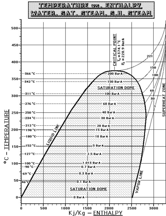
These graphs are NOT useful for sub-cooled liquids; they are ONLY useful for analyzing boiling (vaporizing) liquid/vapors and superheated vapors.
