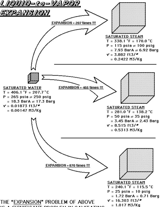
THE “EXPANSION” PROBLEM OF ABOVE IS A SIGNIFICANT PROBLEM IN CAVITATING OR FLASHING LIQUIDS !!!
