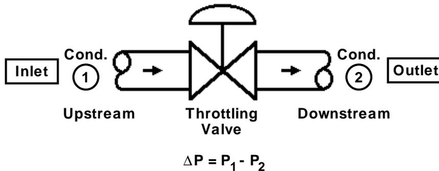
Such valves experience internal velocity and internal pressure gradients (both positive and negative) that conclude with a permanent pressure loss ( $\Delta P$ ) from the inlet pipe-to-outlet pipe connections. Throttling valve trim (plug-seat) experiences relatively high internal velocities nearly 100% of operating time. In comparison, ON-OFF automated or manual valves experience velocity changes ONLY when being actuated from “open-to-closed”, or vice versa; i.e. a few seconds or minutes.
