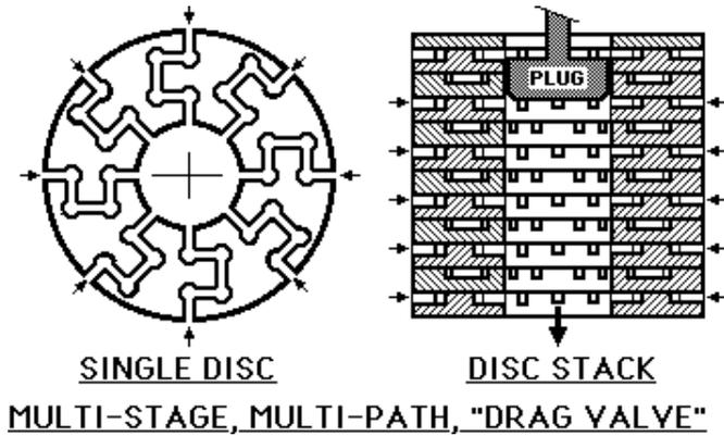
Such drag valves can normally be designed to eliminate cavitation, or at least minimize it. This valve design is very, very expensive and is normally applied in only the most “severe service” instances.
