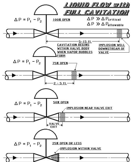
Cavitation is caused by internal fluid pressure conditions, and not by flow rate. As depicted at right, cavitation “moves” around within a valve or its
