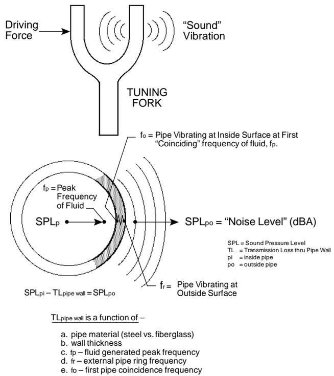
Note: If  $f_p \approx f_r \approx f_o$ , “noise” level is at worst, as destructive wave interference is maximized!
