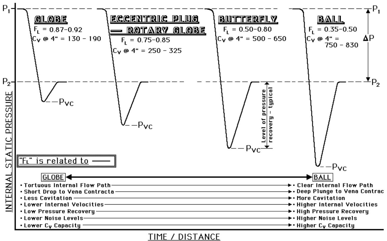
Both butterfly and ball valves are sub-classified as “high recovery valves”. As a general rule, globe and eccentric plug (rotary globe) styles tend to make “better” throttling control valves.
