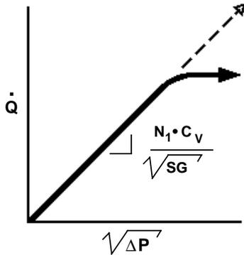
The deviation results because vapor bubbles are forming within the flow
