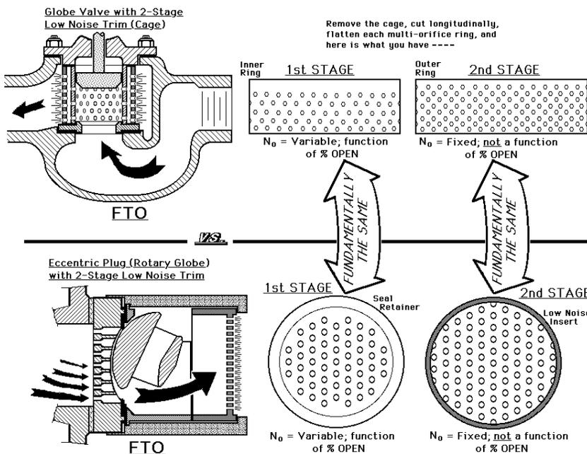
directly from the Cashco factory.) Basically, throttling valve gaseous noise is controlled much as liquid cavitation is controlled by —
