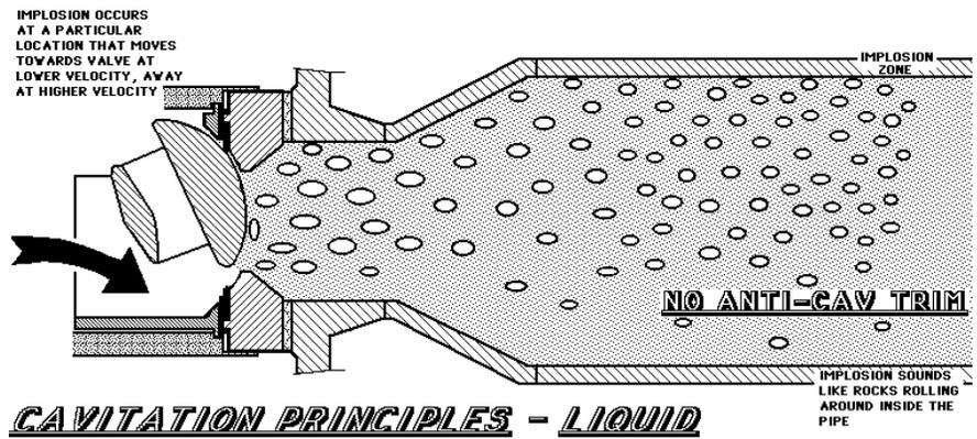
**Physical Mechanism.** The “implosion” of vapor bubbles causes no harm (except vibration) when in the middle of the flow stream. However, when the collapse occurs at the pipe wall, body
