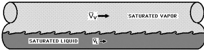
$\bar{V}_{L\&V} = 30-50 \text{ ft/sec}$  **PROPERLY SIZED PIPE** **NO "WAVE" FORMED**
