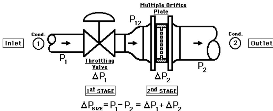
**Reducing Cavitation.** Most “anti-cavitation” throttling valve trim is somewhat of a misnomer. Such trim provides “multiple orifices” that are blocked-off or uncovered as the valve plug travels. This multiple orifice method still produces cavitation but it develops smaller vapor bubbles within the fluid stream. Thus, when the smaller bubbles implode —
