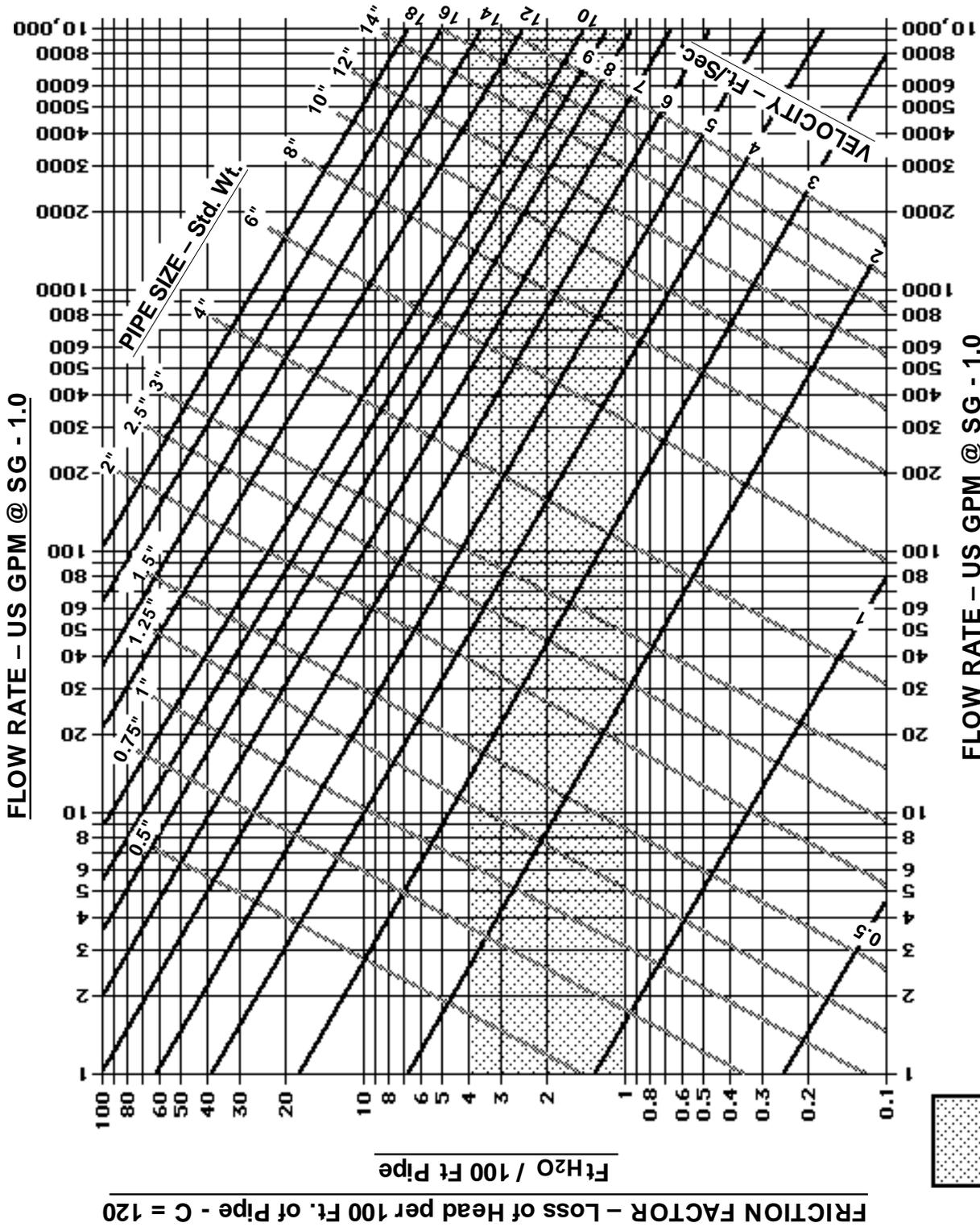
**DETERMINING PIPE SIZE & VELOCITY - LIQUID**
