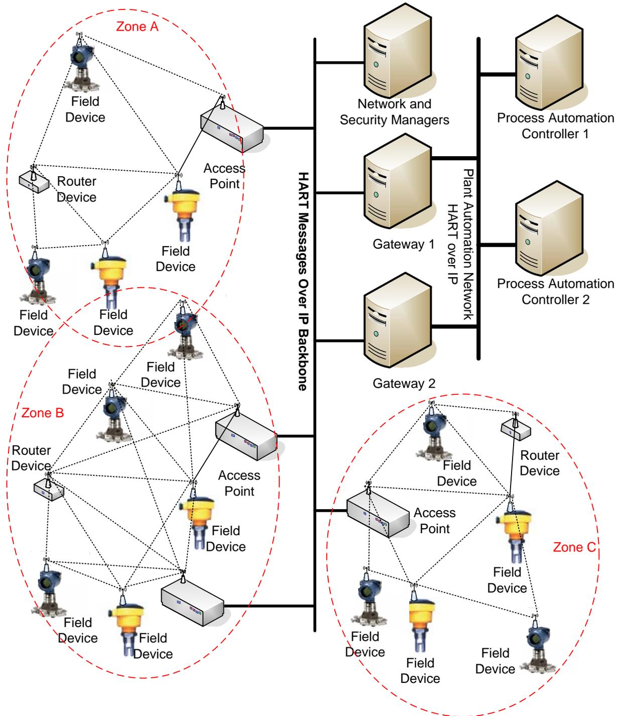
**Figure 2 – Using a single backbone to connect multiple access points.**
