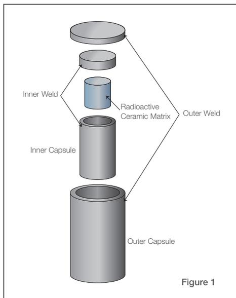
For process level and density measurements, whether the isotope is cesium-137 or cobalt-60, the radioactive materials are inside of a double encapsulated stainless steel cylinder, an example of which is shown in Figure 1. The gamma energy emitted from these capsules does not make an object or person radioactive due to the fact that gamma energy largely passes through objects and people. Some energy will be lost via Compton scattering as the rays pass
