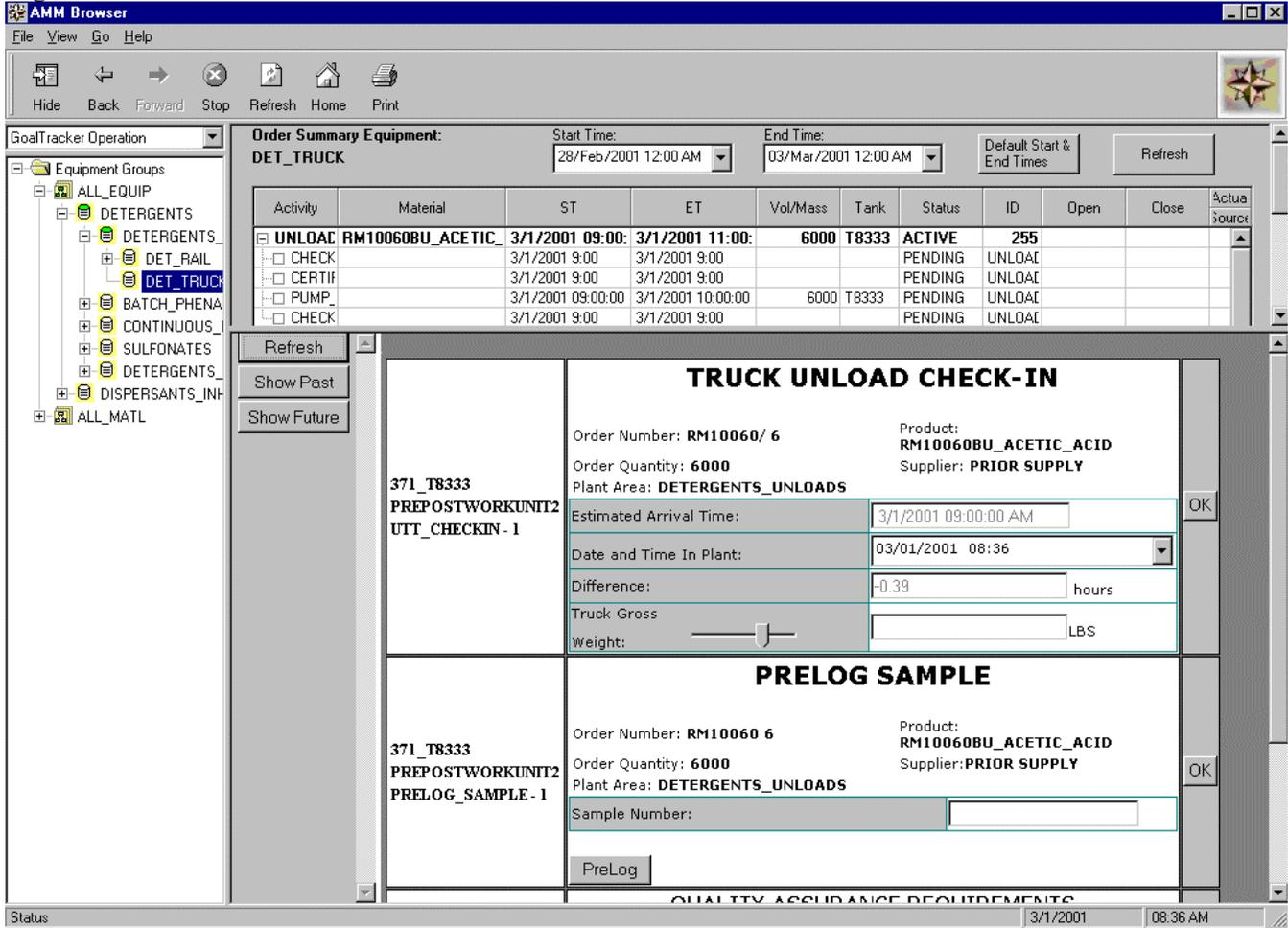
**System Tracking and Optimization** As shown on the software architecture diagram, the integrated historian will consolidate the process, event, and LIMS data for the automated and manual processes. All work procedure events will be automatically recorded with appropriate attributes and time stamps. This will provide Chevron with the environment to analyze and optimize the processes.
