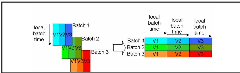
Figure 1: Unfolding approach
