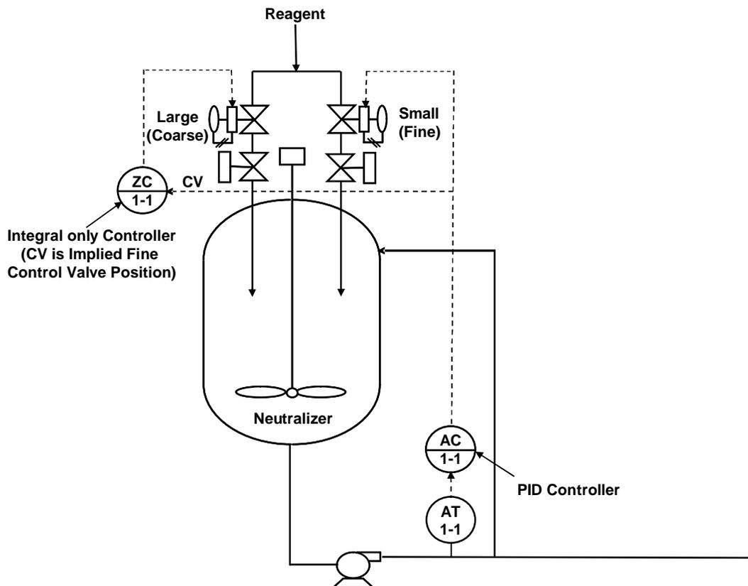
Figure 2 Valve position controller for a neutralizer
