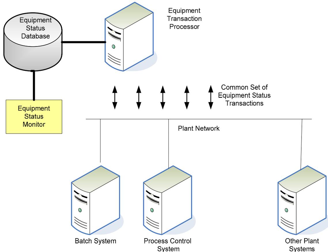
Figure 2 – Equipment Status Architecture
