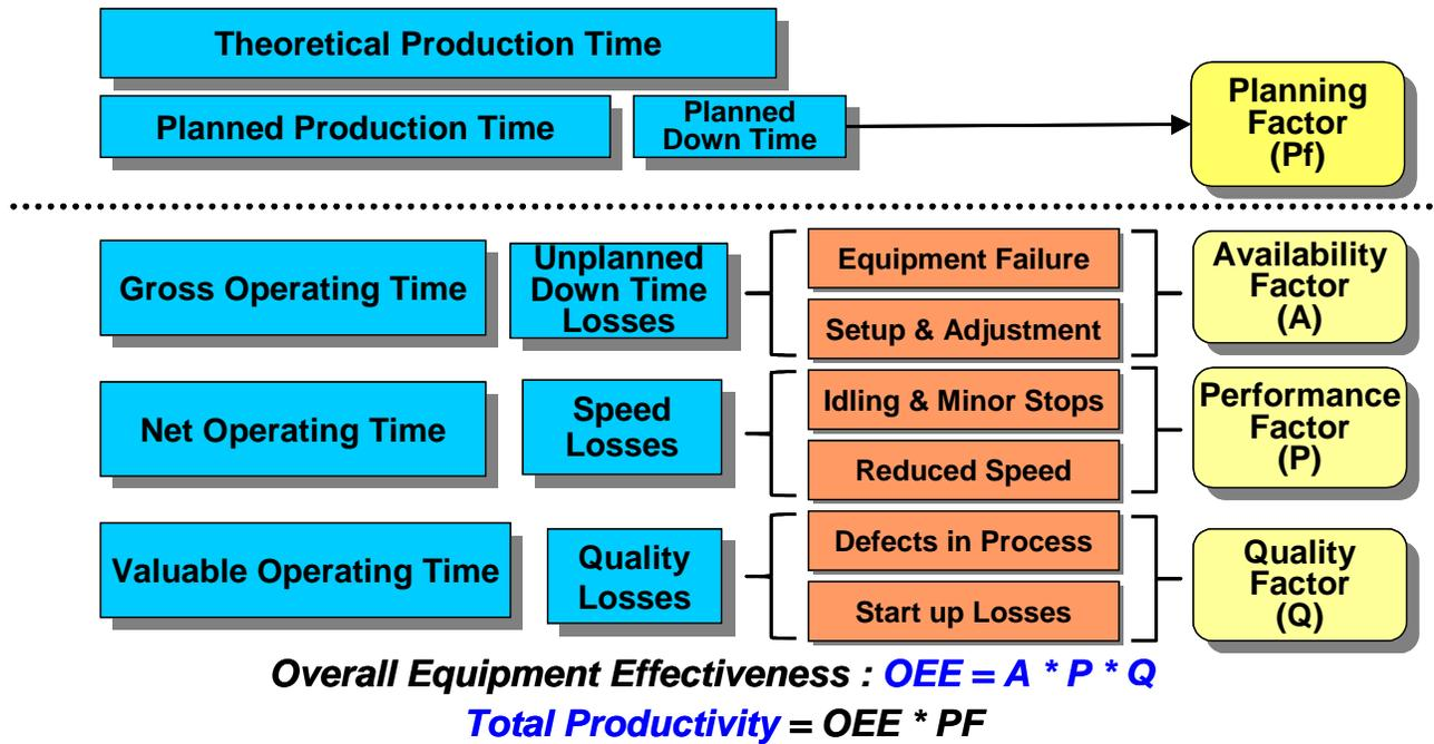
The concepts presented in this paper focus on reducing Equipment Failure, Set-up & Adjustment and Defects in Process. The impact that OEE can have on the financial performance of an organization can be seen in the following figure. Making very modest improvements in OEE can result in a dramatic improvement in financial performance as shown below
