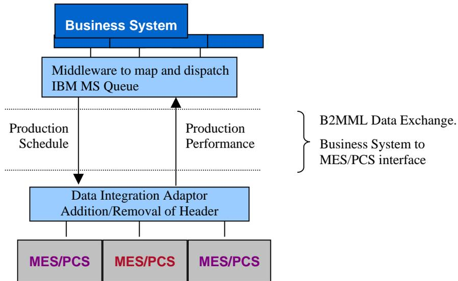
Figure 6: the architecture after the deployment of the ISA S95 standard and B2MML schemas
