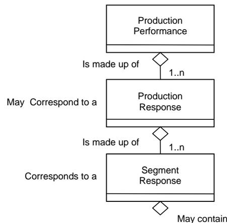
FIGURE 2: Part of the object model of the Production Performance
