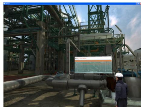
FIG. 4: Augmented reality: example of transparent units for a visual direct feedback on process behavior
